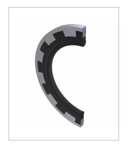
The Parker WO composite sealing washer consists of a metal washer and a circular elastomer sealing lip with an additional mechanical connection to the inside edge of the supporting washer. The serrations achieve a positive connection of the elastomer with the supporting washer and the phenomenon of sheared sealing lips which is frequently encountered with composite seals is prevented.
