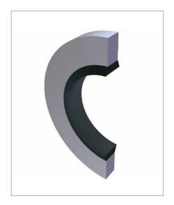
The WX Parker composite sealing washer consists of a metal washer with a rectangular cross-section and an elastomer sealing lip with a trapezoidal cross-section that is vulcanised to the inside.
