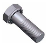
Parker WO series composite sealing washers are designed for radial sealing below the screw head in the area of the smooth (non-threaded) screw shaft. This provides three functionally relevant sealing areas. The elastomer sealing lip is mechanically connected to the metal carrier.
