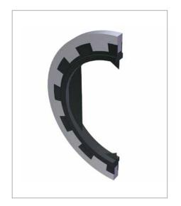
The Parker WO composite sealing washer consists of a metal washer and a circular elastomer sealing lip with an additional mechanical connection to the inside edge of the supporting washer. The serrations achieve a positive connection of the elastomer with the supporting washer and the phenomenon of sheared sealing lips which is frequently encountered with composite seals is prevented.
