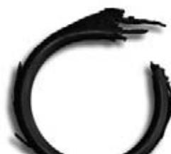
Fig 9.6 Extruded O-ring
