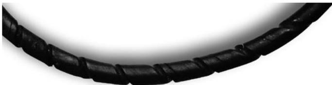
Fig. 9.10 Twisted O-ring with spiral marking
