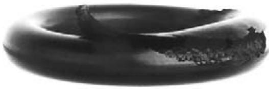
Fig. 9.8 Peeled O-ring
