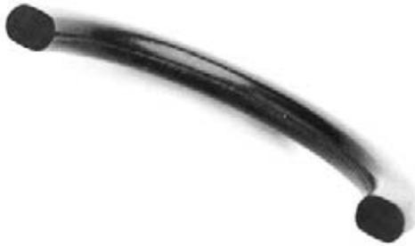
Fig. 9.9 Characteristic compression set. High deformation
