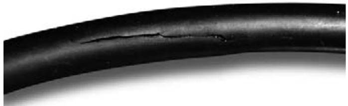
Fig. 9.12 O-ring damaged by explosive decompression
