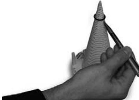
Identification of the 2-xxx size number with the measuring cone
