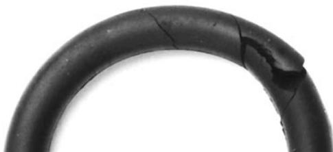
Fig. 9.11 Twisted O-ring with spiral cuts in surface
