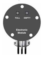
Red wire to ignition power (12 or 24 volt). White wire to existing send wire off old sender. Black wire to existing ground wire off old sender.
