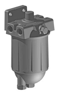
The Racor 110A fuel filter/water separator features a variety of compact sizes to fit the most cramped engine compartments. All units feature 1/4"-18 NPTF inlet and outlet fuel ports and a unitized mounting bracket.
