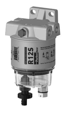
The Racor 120A fuel filter/water separator features a variety of compact sizes to fit the most cramped engine compartments. All units feature 1/4"-18 NPTF inlet and outlet fuel ports and a unitized mounting bracket.
