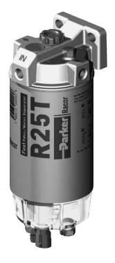
All 200 Series filters feature Spin-On, high-capacity, Aquabloc®II replaceable filter elements which separate water, remove solid contamination, and are available in 2, 10, and 30 micron.
