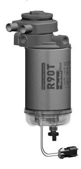
Racor's 300RC Series Fuel Filter/ Heater/Water Separators are specifically designed to handle today's tough fuel system problems. These units feature a standard high efficiency coolant heat exchanger to heat incoming fuel and are only different in flow capacity and element size.
