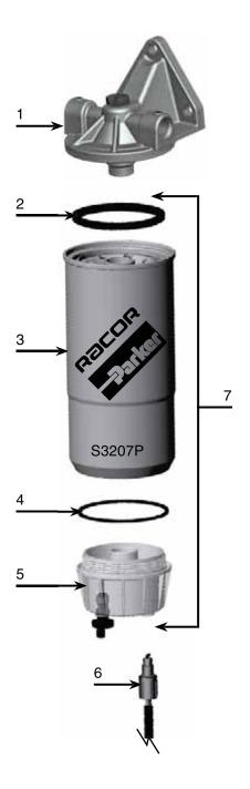
The standard B32007 bowl has no water sensor port. Bowls with water sensor ports are available as replacement kits (see item #5 above). Do not use water sensors on gasoline applications.
