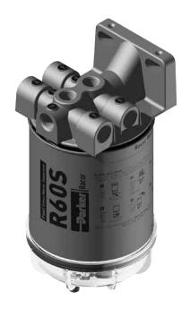
All 600 Series Spin-On fuel filter/water separators feature multiple fuel ports (4 inlets and 3 outlets) and a unitized mounting bracket for installation convenience. Inlet and outlet threads are 3/8"-18 NPTF for all models. These filter assemblies provide flexibility during mounting and fit any engine application.
