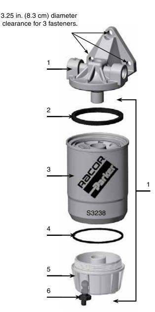
The standard B32038 bowl has no water sensor port. Bowls with water sensor ports are available as replacement kits (see item #5 above). Do not use water sensors on gasoline applications.
