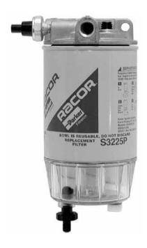
Racor's 325R Diesel Fuel Filter/ Heater/ Water Separators are specifically designed to handle todays tough fuel system problems. These units feature a standard in-head PTC heater and reusable see-thru contaminant collection bowl. They are different only in flow capacity and element size.
